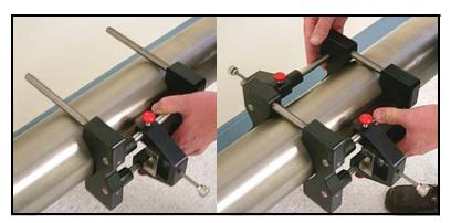
Figure 3-7: Mounting the Two Halves of the Fixture
